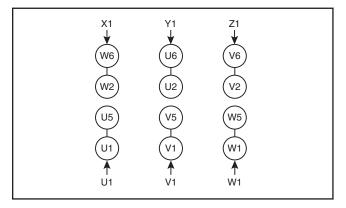
Figure 54. 220V motor wiring.
